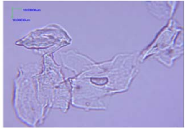
2000X NorGraphene graphene (10 μm scale)
